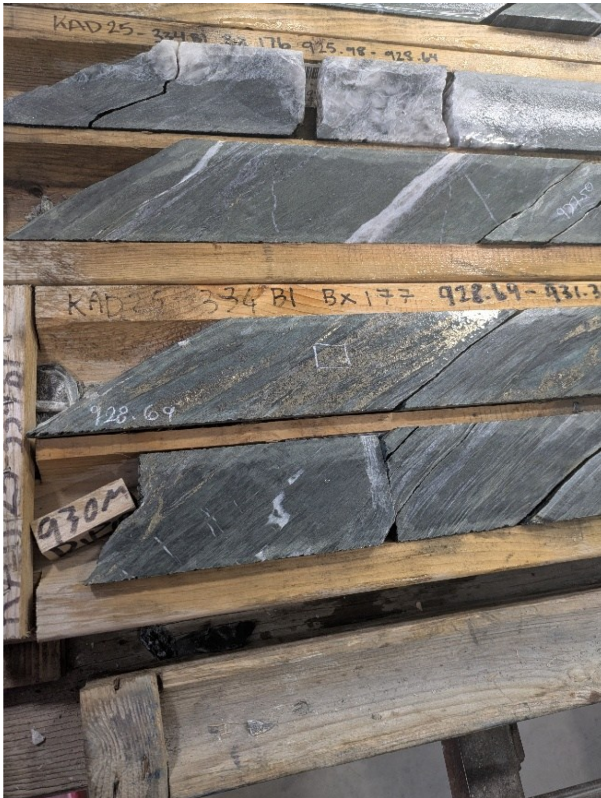
Figure 12.5: Sulfide Mineralization in Geminid Drill Core
