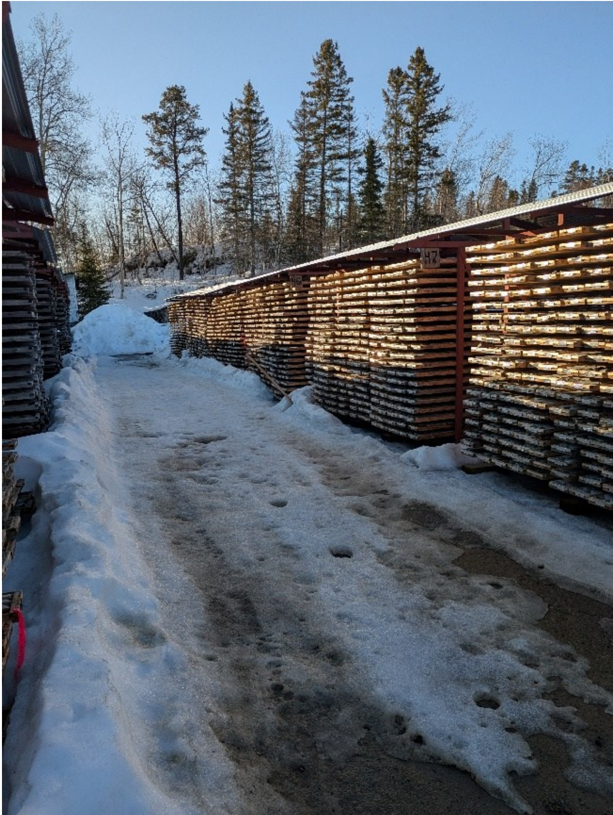
Figure 12.3: Core Storage Facility
